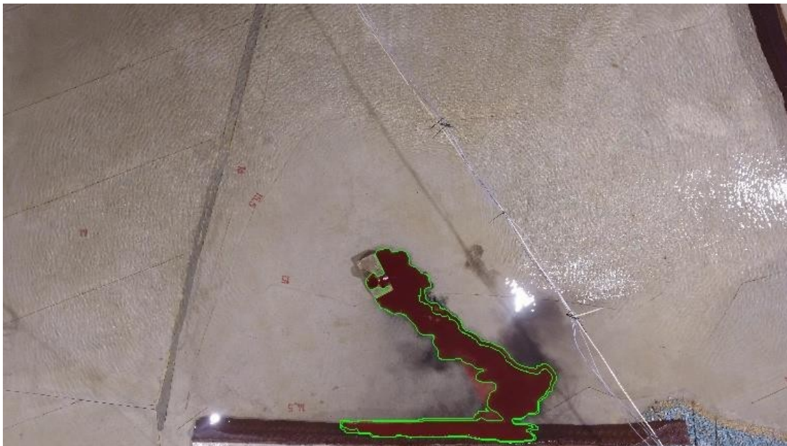
Figure 1: WBreeze algorithm's result of detection and tracking the oil spill during the testing in the CAMERI pool.
